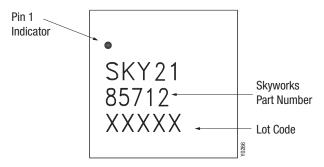
Figure 6. Typical Part Markings (Top View)
