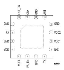
Figure 2. SKY85712-21 Pinout (Top View)
